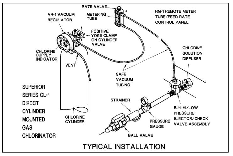
SPECIFICATIONS The chlorinator shall be SUPERIOR™ MODEL CL-1 manufactured by Chemical Injection Technologies, Inc., Ft. Pierce, Florida, and shall have a maximum capacity of \_\_\_\_\_ pounds per day (gr/hr)of chlorine feed and shall be equipped with a chlorine flow meter of pounds per day (gr/hr)
