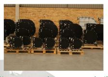
Above is a picture of a recent contract for 48 pumps of various sizes L25 to L100, selected for the applications, because of the L Series high flow per revolution and longer hose life.
