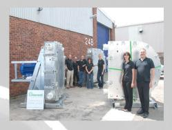
3 off L150 pumps on a thickener underflow application, chosen due to its high flowrate and low power consumption. As well as saving on power, our low friction rollers dramatically reduce wear on the hose caused by the physical stretch and frictional heat from competitors fixed shoe designs, greatly extending overall hose life.
