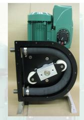
L15 with cover removed, showing its smart roller design which applies a low friction soft compressing action, compared to our competitor's high friction rubbing shoe. The L15's proven roller design also imparts minimal stretch and heat input to the hose, doubling hose life and significantly reducing power consumption.
