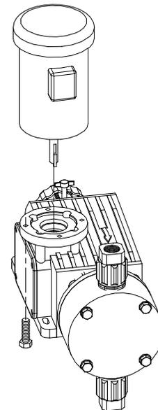
*Figure 11, motor mounting*
