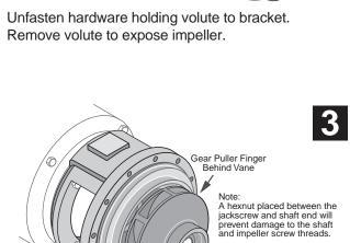
Install a standard gear puller to shaft end and impeller, placing puller fingers behind impeller vanes as shown.
