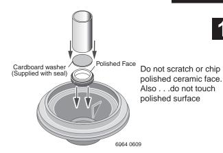
Place seal plate on a smooth, flat surface, pump side up.
