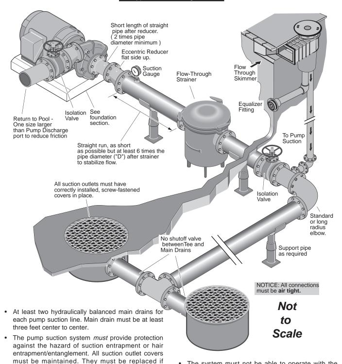
The system must not be able to operate with the pump drawing water from only one main drain (that is, there must be at least two main drains connected to the pump whenever it is running.) However, if two main drains run into a single suction line, the single suction line may be equipped with a valve which will shut off both main drains from the pump.
