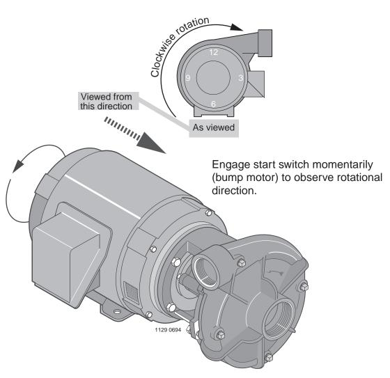
Direction of Pump Rotation is determined by viewing liquid end of pump from the **back** or **shaft side**, and **not** from looking into the impeller eye or front of volute case. A rotation direction arrow is cast into the pump body and shows correct rotation.
