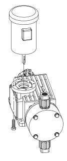
Figure 11, motor mounting
