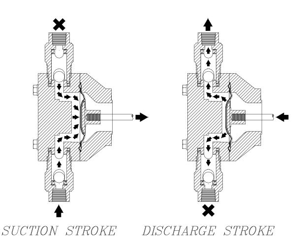
Figure 1, reagent head operation
