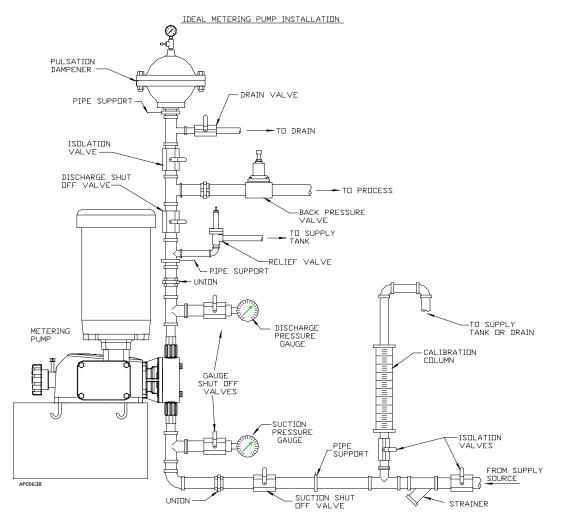
Figure 3, sample system configuration
