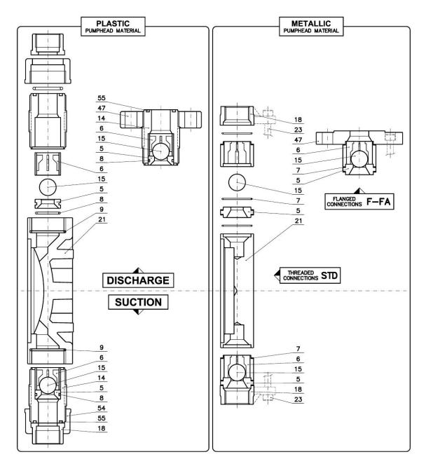
Figure 9, check valves to 137 GPH
