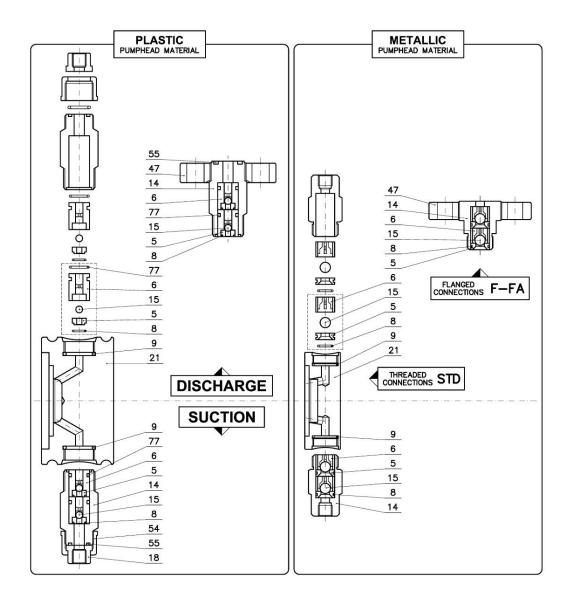
Figure 8, check valves to 60 GPH
