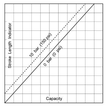
Figure 6, sample flow calibration curve
