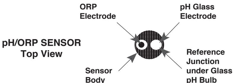
Leaving high pH (alkaline) solutions in contact with the pH sensor for long periods of time is harmful and will cause damage. Rinsing such liquids from the pH/ORP sensor well and refilling it with Myron L Storage Solution, a saturated KCl solution, pH 4 buffer, or a saturated solution of table salt and tap water, will extend the useful life.
