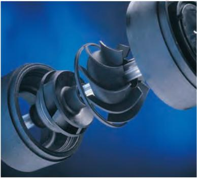
The SQ/SQE pump design uses "floating" impellers. Each impeller has its own tungsten carbide/ceramic bearing. This design and the high quality of materials make the pump very wear resistant.
