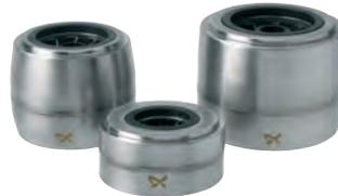
Internal leakage caused by pressure differentials within the pump was minimized. Tests have shown that an impeller seal clearance gap of just 0.4 mm between the impeller and the chamber causes a 5% drop in efficiency. When liquid seeps out into the pump, precious energy is wasted on circulating that liquid. Grundfos uses a floating seal ring between chambers, providing a nearly perfect seal.
