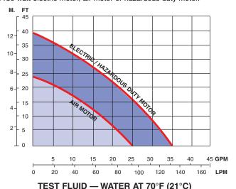
Flow curve for **Stainless Steel Pump Tube** with electric motor, air motor and hazardous duty electric motor.
