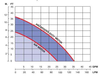
TEST FLUID — WATER AT 70°F (21°C)
