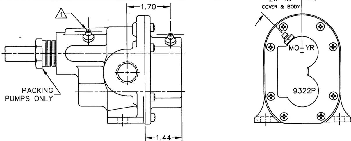
⚠ GREASE FITTINGS (ITEM 17) INSTALLED INTO .125-27 NPT CONNECTIONS.
