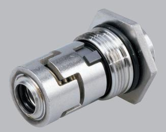
The patented Grundfos cartridge design ensures that the seal components will never be assembled wrongly, the spring will never be incorrectly preloaded, and that sensitive surfaces will never be subjected to greasy fingers or dirt. All these factors are common causes of short seal lifetimes in other pumps.
