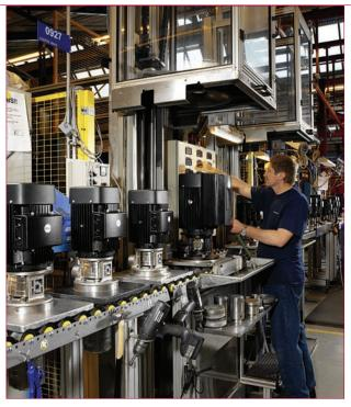
Assembly line of immersible pumps at Grundfos.
