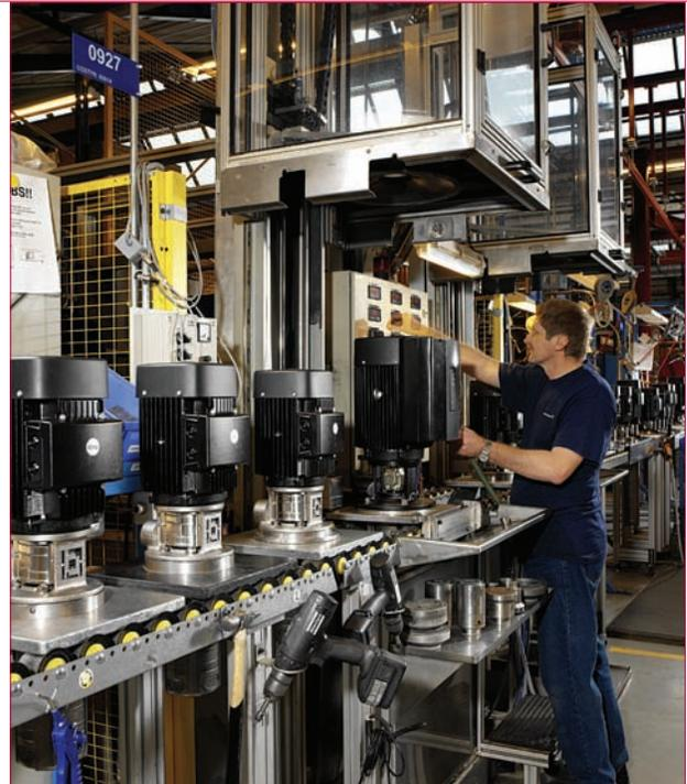
*Assembly line of immersible pumps at Grundfos.*
