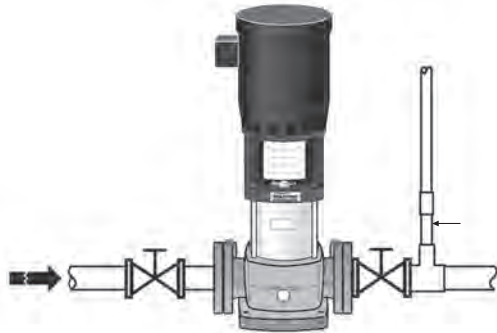
Fig. 7 Recommended bypass arrangement
