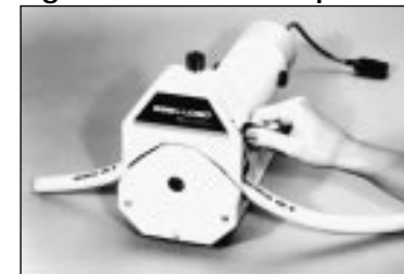
Figure #3. Close Pump
