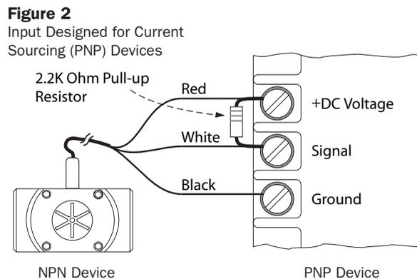
Since the three-wire pickup sensors are solid state, they do not exhibit switch bounce and can be used at relatively high frequencies.
