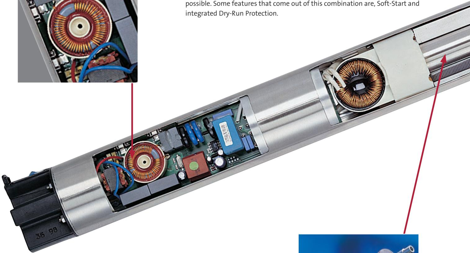
The SQ and SQE motors are based on a permanent-magnet rotor which produces high efficiency output within a wide load range. Other benefits include reduced heat production and start-up torques comparable to 3-phase motors, in a simple-to-install 2-wire format
