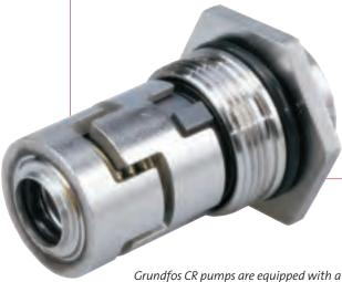
Grundfos CR pumps are equipped with a unique, easy-to-replace cartridge shaft seal that's available in a choice of materials. It can handle temperatures from -40°F to 250°F (consult factory for complete booster systems when the operating temperature is greater than 176° F).
