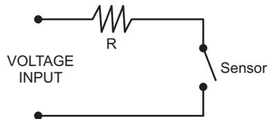
High surge currents may cause damage to the sensor and significantly reduce its life, the following circuit is, therefore, highly recommended.
