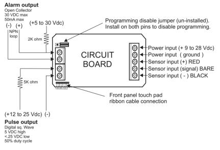
NOTE: To reset the circuit board: 1) Disconnect power 2) Apply power while pressing the two front panel buttons.
