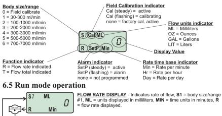
FLOW TOTAL DISPLAY - Indicates accumulated total flow, S1 = body size/range #1, ML = units displayed in milliliters, T = total accumulated flow displayed.
