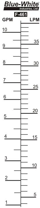
Read Float at Top Liquid - Sp. Gr. 1.0 Calibrated with Water Model # F-461100LX
