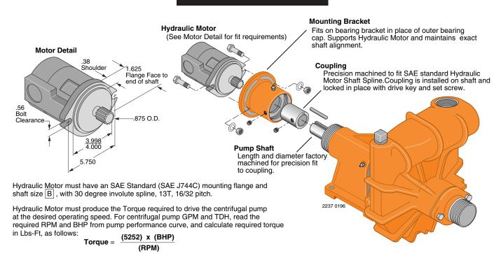
Hydraulic Motor selected must match with the flow and pressure capability of the hydraulic power source system. The operating speed of the centrifugal pump will be controlled by the valves in the hydraulic power source system.
