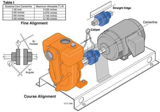
AWARNING Rotating shaft can catch and trap clothing or body. Coupling guard must ALWAYS be in place when pump is running. Coupling guard shown in phantom for pictorial clarity.
