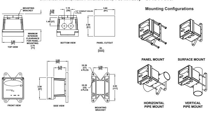
SHARK-TX Universal Mount, NEMA 4X Enclosure, 4-20 mA Loop + 24 VDC Power
