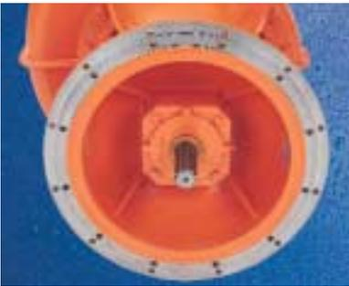
**SAE #2 or #3 engine versatility** – Pre-drilled mounting holes allow for maximum engine-choice flexibility.
