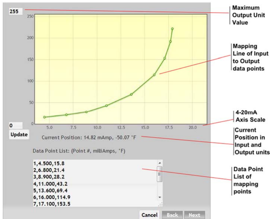
Figure 6-6 - Non-linear scaling window. One must enter the calibration points manually into the bottom text box. This example shows a true non-linear scaling though this “non-linear” scaling can also be done for a linear output sensor.
