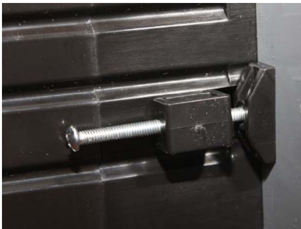
Figure 2-1 - Mounting hardware attached to panel with 4 in-lb of torque
