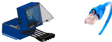
Connect the RJ-45 cable to a router or cell modem with an internet connection. The *MicroVision<sup>EX</sup>* will automatically detect and assign an IP address and will connect to [www.PULSAlink.net](http://www.PULSAlink.net) automatically.
