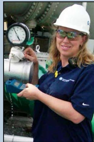
The 6Pfc measures a dynamic range of free chlorine concentrations wider than the range of colorimetric test kits.
