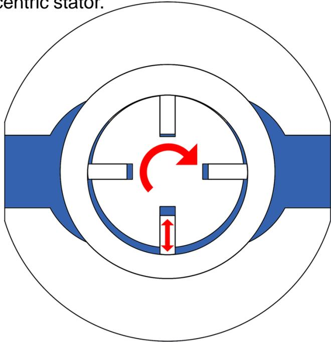
According to the positive displacement principle, these sliders generate a nearby pulsation free flow with high discharge pressure and low flow rates.
